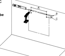
STEP 2. Install the cabinet on the drilled holes
