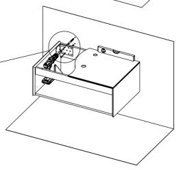
**STEP 3.** Fill the side against the wall with Silicone and finish
